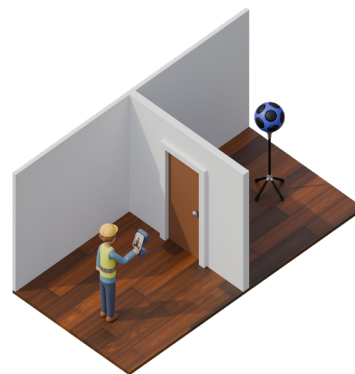
Image 2 - How to visualize leaks on indoor walls during construction
